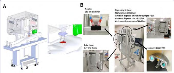
**Figure 3:** A) Schematic illustrating scale, design and component of *in situ* bioprinter for wound regeneration. B) Primary components of an in situ bioprinter, including 260 μm diameter nozzles, driven by up to 8 independent dispensers connected to a print head with XYZ movement system, and 3D wound scanner. Reproduced with permission [99]. Copyright 2019, Springer Nature.
