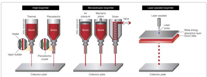
Figure 1: a) Inkjet bioprinter: A pulse thermal or piezoelectric stimulus causes fine droplets of bioink to be emitted from the nozzle. b) Microextrusion bioprinter: A stream of bioink is deposited in response to pressure exerted on the reservoir. c) Laser assisted bioprinter: A pulsed laser beam is directed at a band of metal which absorbs and transmits the energy to the bioink present underneath.
