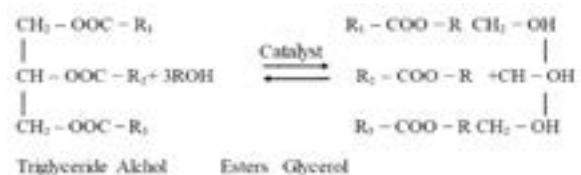
Figure 2: Chemistry of esterification.
