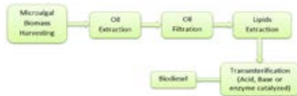
Figure 1: Microalgal biodiesel production pathway.
