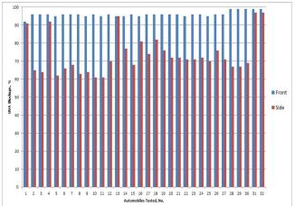
Figure 4: The distribution of front windshield UVA blockage compared to distribution of side window UVA blockage for same vehicles.
