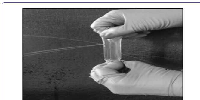
Figure 1: Perforation in dialysis tubing: The crude fungal extract was precipitated with solid ammonium sulphate (see methods). The extensive dialysis resulted in the formation of pores in dialysis tubing due to cellulase action. Note the loss of sample from dialysis tubing when squeezed downwards.
