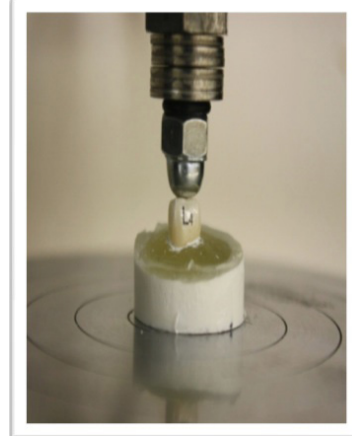
Figure 1: Die-crown unit placed in a universal mechanical testing machine.
